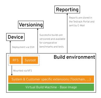
Embedded systems need to provide SSH access in order to be enabled for automated build and test services. This can be done in advance, or when the hardware is installed, via the browser based Testrack Portal with the serial console.
